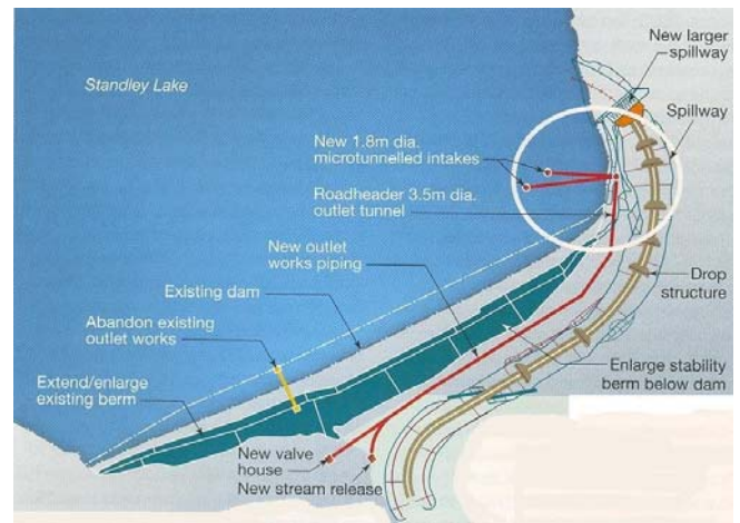
Figure 31. The Standley Dam Rehabilitation project (Coss, 2006).
